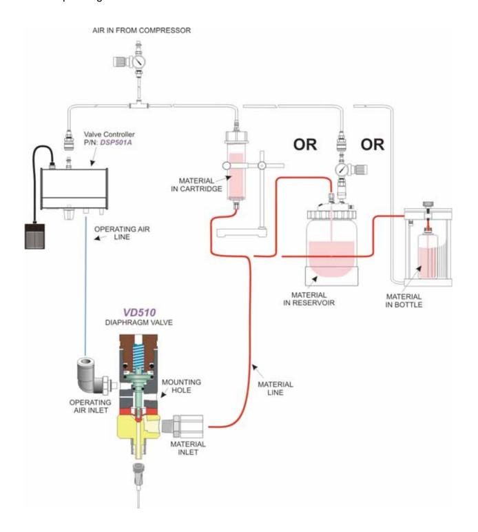
**5-1-1)** Fasten the valve firmly using mount hole. (M5\*P0.8\*D98)
