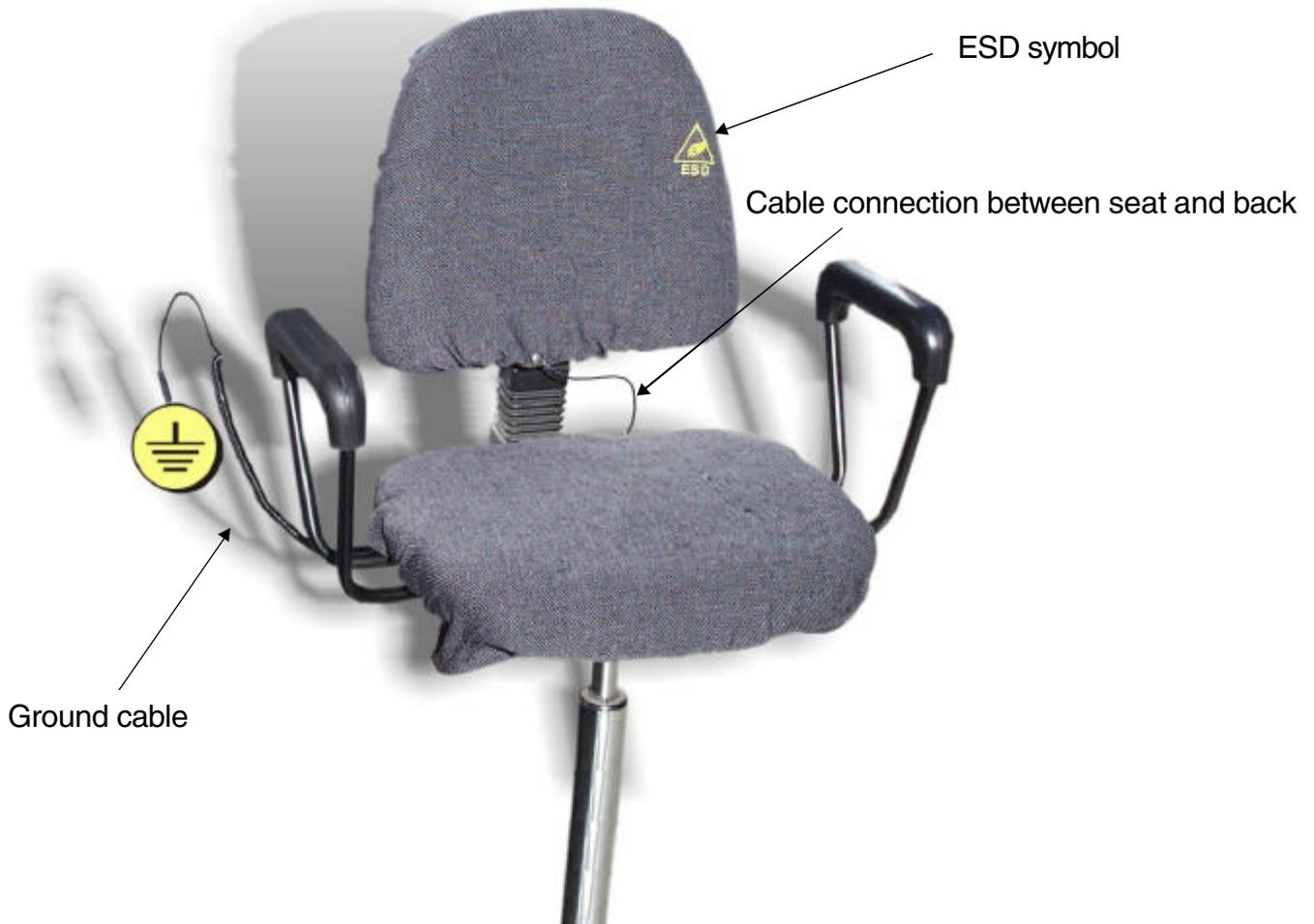
Made of gray conductive woven fabric, the dissipative chair covers are designed to make a conventional padded factory chair more suitable for use in EPA. The covers easily fitted on all chair types, are supplied with the cables to connect the backrest to the seat and the seat to the ground.
