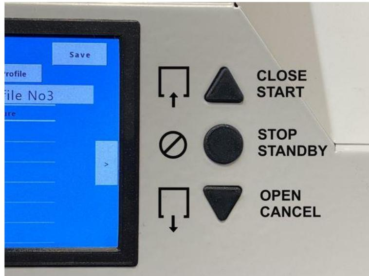
**"CLOSE/START" button** - Button to start the motor that closes the door.
