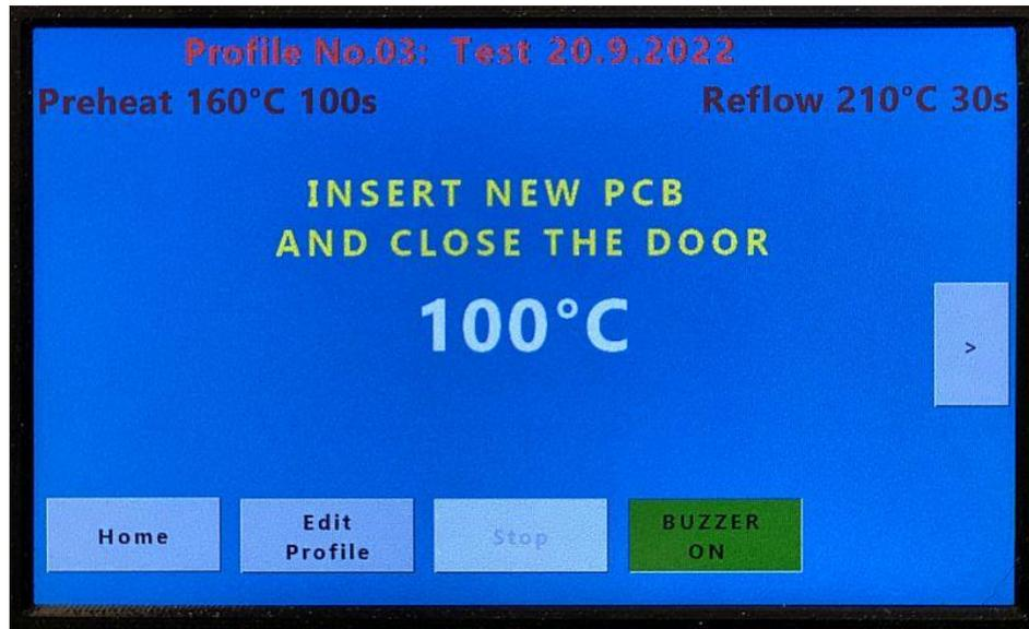
After the end of cooling, the oven prompts us to insert the PCB and the normal cycle begins according to selected or edited profile as described in chapter 6.1
