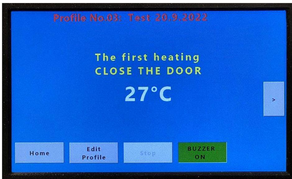
Immediately after that, the oven prompts us to close the door with the HW button "CLOSE" and after closing, the first heating cycle begins. The oven starts to heat up to a temperature of 200°C and when this temperature is reached the door opens automatically and the oven cools down to an initial temperature of about 100°C.
