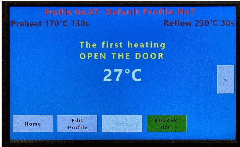
Pressing the "HEAT UP START" button will start the first heating cycle and the oven will ask us to open the door fully (100%) to calibrate the limit switch. We open by pressing the "OPEN" hardware button.
