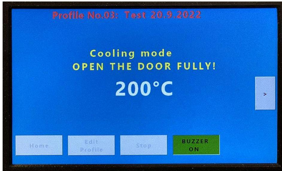
You can end the running program at any time by pressing the "Stop" button. We also end the program by pressing the "OPEN/CANCEL" control button. see chapter 4.
