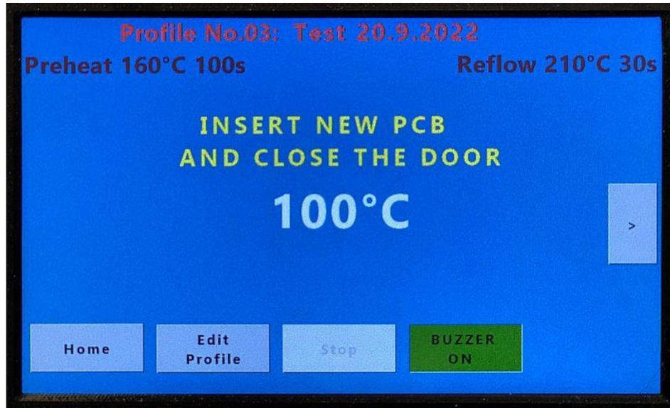
As described in chapter 4, the currently selected or last used profile is activated after the door is closed. Immediately after turning on the oven, the last profile used before turning off the oven is set.
