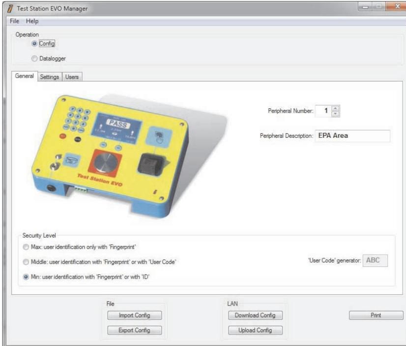
Peripheral Number: it's a unique number ID (from 1 to 100) that identify the TestStation. It's possible to use till 100 Test Station in a factory and "merge" the data collected from them.
